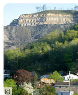
(c) With mountaintop removal, everything lying above an ore deposit is just removed. This controversial mining technique is common in coal mining regions, such as Kentucky above.
